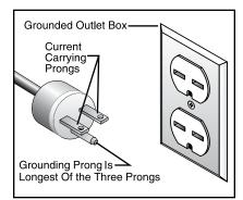
Figure 1. Ground plug configuration.
